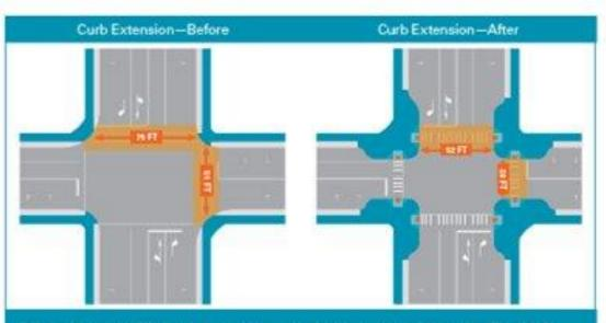
Carb extensions improve visibility for pedestrians and drivers, reduce the pedestrians crossing distance, calm traffic, and shield on-street parting at intersection approaches. In the above example, the addition of ourb extensions shortens pedestrian crossing distances from 75 feet to 52 feet in one direction and 51 feet to 28 feet in the other direction without reducing the number of travel lanes.
