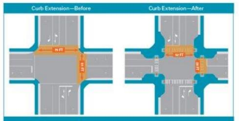
Cerb extensions improve visibility for pedestrians and drivers, reduce the pedestrian crossing distance, calm traffic, and shield on-storet parting at intersection approaches. In the above example, the addition of ourb extensions shortens pedestrian crossing distances from 75 feet to 52 feet in one direction and 51 feet to 28 feet in the other direction without reducing the number of travel lates.
